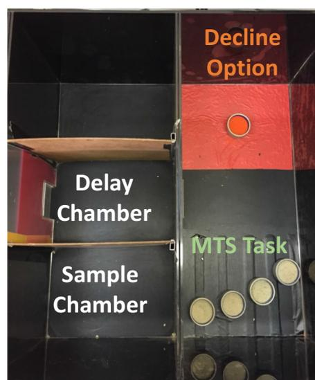
**Fig. 1** Photograph of the testing apparatus, which was divided into the *sample chamber*, *delay chamber*, and *testing chamber* (on the right). The testing chamber was divided into two sides: (1) the decline option area, which was bumpy in texture and covered in red contact paper, and contained the decline cup and (2) the MTS task area, which was corrugated in texture, covered with black contact paper, and contained the four choice cups
